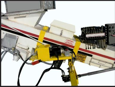
The Conveyor Mounted Door Demon® features smooth hydraulic pressure for maximum torque to open even the toughest hopper gate doors. The unit is self-contained so it does not affect the conveyor's functions. The Conveyor Mounted Door Demon® can be mounted in the left- or right-hand position and exhibits total product flow control with smooth hydraulic height adjustment for varying capstan levels.
